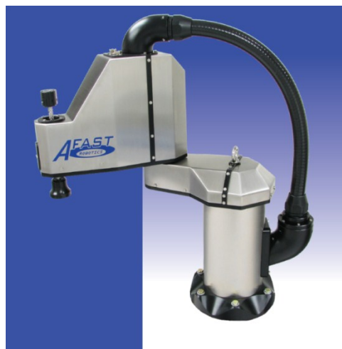
Slika 2.13: Open platform SCARA robot, Afast Robotics
